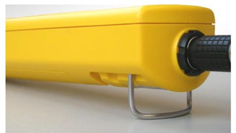
*The optical interface connector and AC adapter / charger connector compartment is sealed with a rubber cap. The tilt stand provided in addition to the tripod bush can be used to place the instrument securely on a flat surface.*
